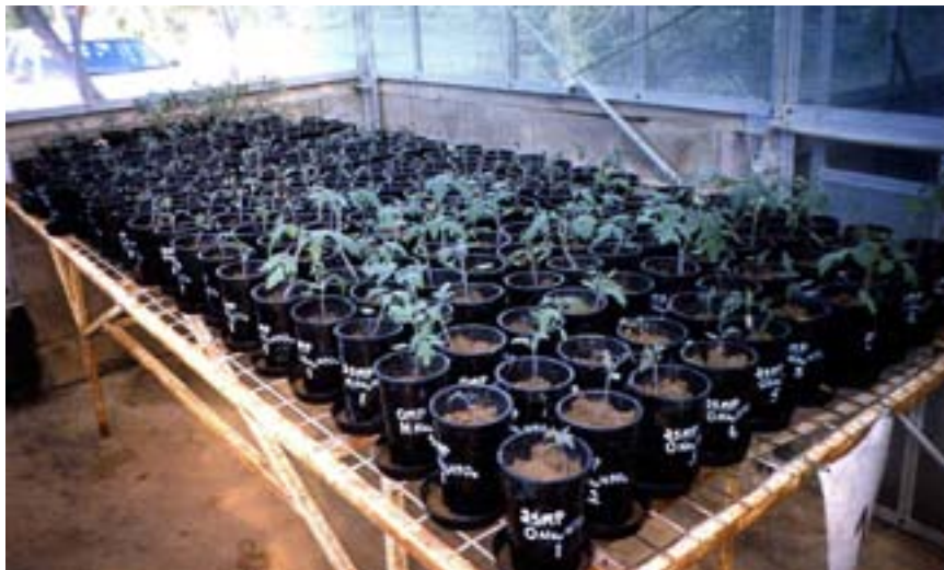
Figure 6.1 Part of the pot trial at James Cook University, Townsville, designed to use relative differences in growth of tomatoes as a bioassessment of the differences in samples of the Innisfail Clay that had been treated with 3 rates of Minplus™ and 4 rates of 4 soil modifiers. The experiment provided the basis for determining the nature of the constraints to plant growth presented by the soil, and the extent to which Minplus™ may overcome those constraints. The pots were arranged in treatment blocks for this photograph, which was taken about half way through the experiment.
